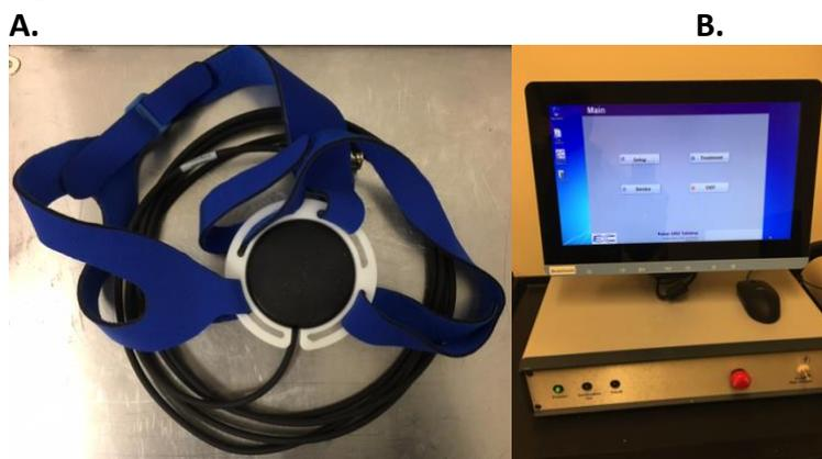
Fig. 1. A) Transducer, housing and head strap. B) Ultrasound console.
